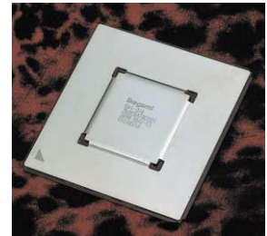
Next-generation digital process ASIC (0.18μm design rule)
