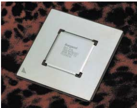
Next-generation digital process ASIC (0.18um design rule)
