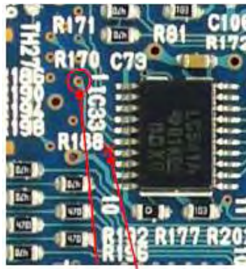
Fig.2 The through-hole and the point to be cut on the printed wiring pattern coming from pin# 7 of IC33
