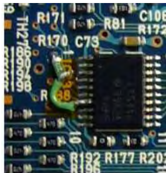
Fig. 3 After the wiring, glue the parts (The factory uses the "Super-X" glue)
