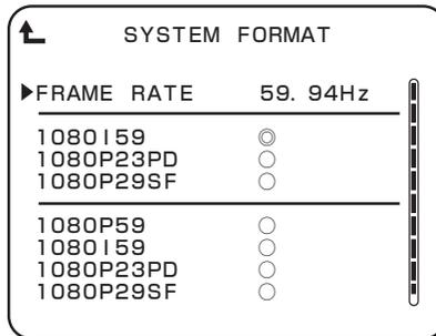
Set the blinking cursor to the format to be set and execute the setting as the mark on the screen becomes "◎".
