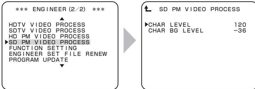
To position the flashing cursor on the "SD PM VIDEO PROCESS", and determine.
