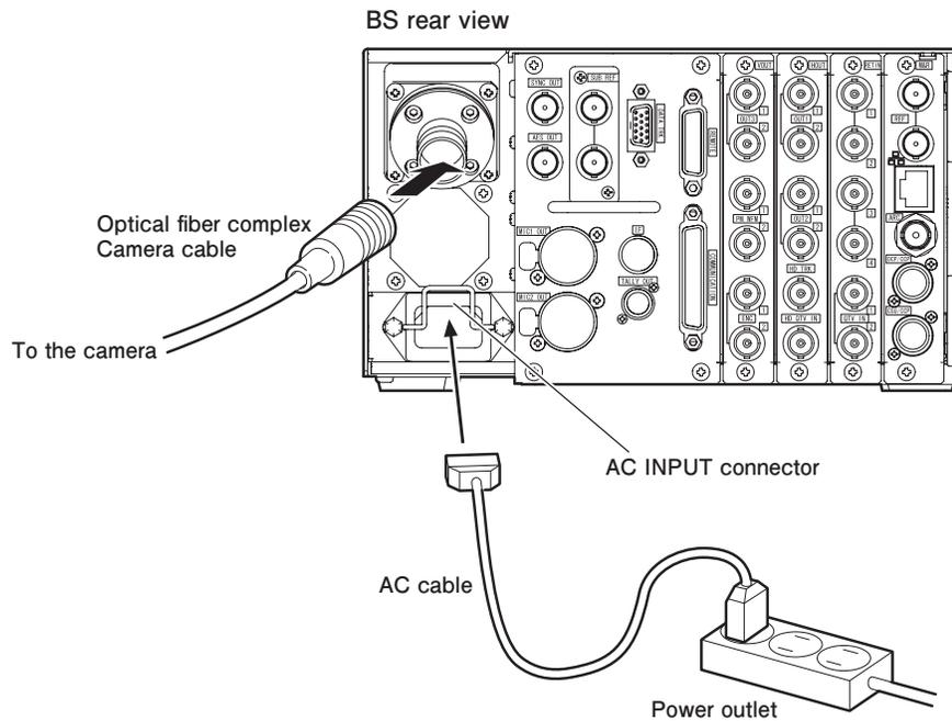
Two methods of power supply to the camera head are available with this configuration.
