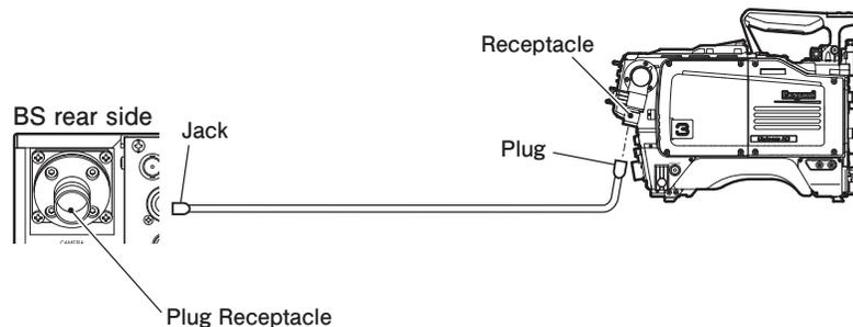
Clean the four sections: receptacle on the camera head, plug receptacle on the BS, and plug/jack on both ends of the camera cable. The cleaning method for male connectors differs from that for female connectors.
