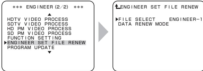
To position the flashing cursor on the "ENGINEER SET FILE RENEW", and determine.
