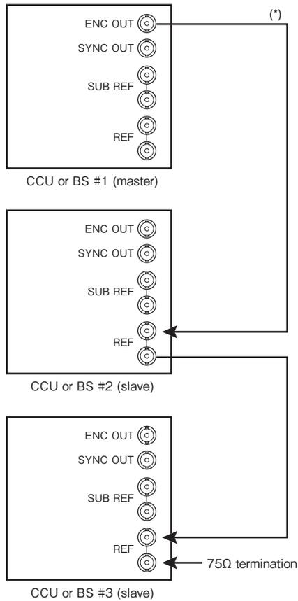
\* In that case, add 10 FIELD ID signal (SMPTE 318M compatible) to the ENC signal output of the master equipment.
