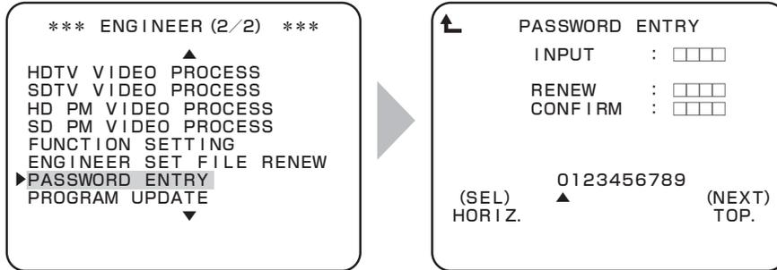
To position the flashing cursor on the "PASSWORD ENTRY", and determine.
