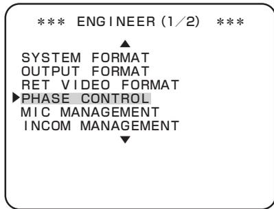
To position the flashing cursor on the "PHASE CONTROL", and determine.
