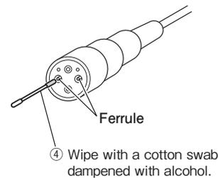
**5** After wiping the Ferrule with alcohol, wipe the Ferrule with a dry cotton swab.
