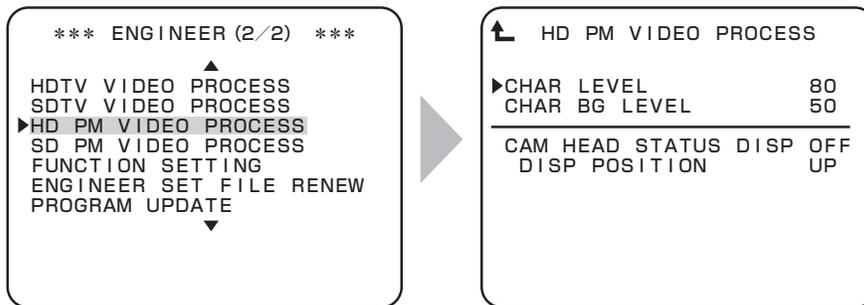
To position the flashing cursor on the "HD PM VIDEO PROCESS", and determine.
