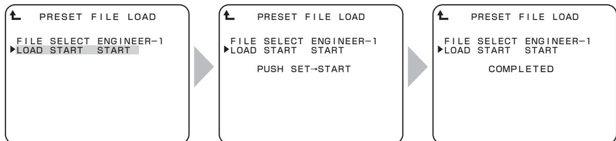
Position the flashing cursor on "LOAD START", and confirm the selection.
