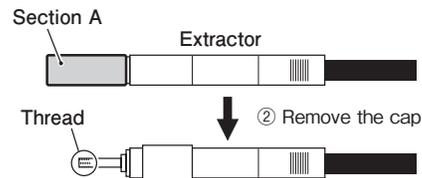
**3** Insert the extractor into the alignment sleeve and turn the extractor clockwise 8 to 10 turns until it stops. When it stops, pull the extractor out straight.
