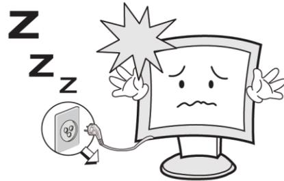
When smoking and noising from the monitor, unplug the product from the wall outlet and contact a service center.
