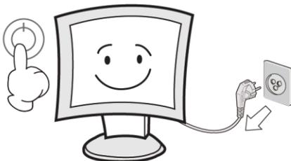
Take the power plug out from the wall outlet. Do not pull the cable. It may snap the inner-wires and cause overheating and fire.
