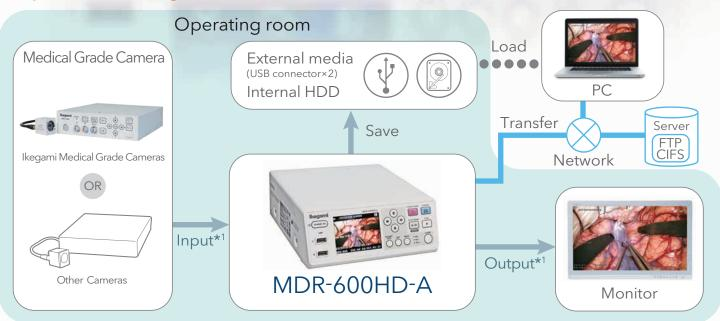
\*1 Digital: SD-SDI/HD-HDI/DVI-D | Analog: Composite/S-Video Input signal and output signal format must be the same
