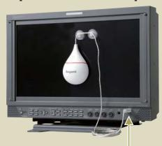
Simply connect the ASP cable to USB interface
