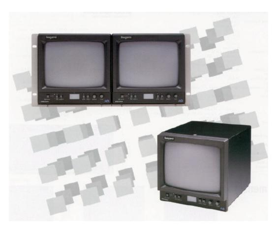
Ikegami's HPM-9050 9-inch high performance monochrome monitor with a high resolution CRT delivers over 800 lines of horizontal resolution. Switching power supply circuitry provides a wider range of supply voltages, while its back porch clamp assures consistent stability for the video black level.
