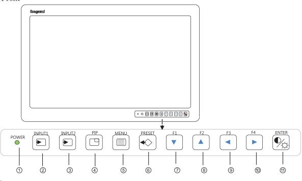
① Power indicator : When the power is in "ON" mode ------ Illuminate in Green
