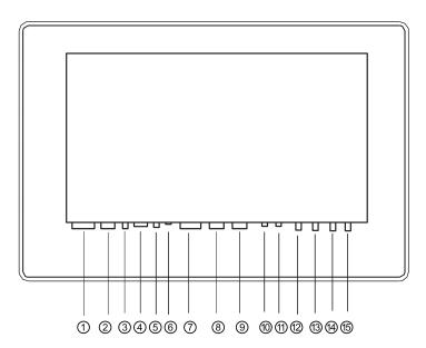
1) Power switch : The power to "on", "off".2) DC input socket : Connect the AC adapter.
