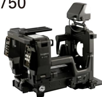
Converting the portable camera (Unicam HD) into a full facility studio camera.
