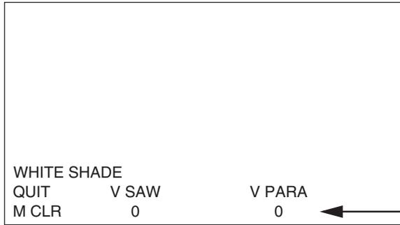
If the MENU switch is pressed while any of "V SAW" or "V PARA" is blinking, the value below it can be changed. Selecting "M CLR" makes the system to be set back to the factory setup.
