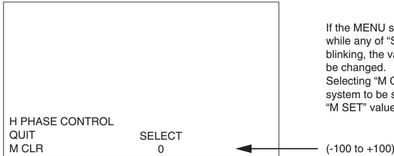
If the MENU switch is pressed while any of "SELECT" is blinking, the value below it can be changed. Selecting "M CLR" makes the system to be set back to the "M SET" value.
