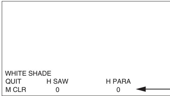
If the MENU switch is pressed while any of "H SAW" or "H PARA" is blinking, the value below it can be changed. Selecting "M CLR" makes the system to be set back to the factory setup.
