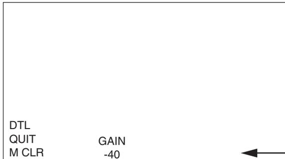
If the MENU switch is pressed while any of "GAIN" is blinking, the value below it can be changed. Selecting "M CLR" makes the system to be set back to the "M SET" value.
